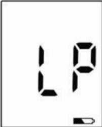
A square icon representing a low power message. It features the letters 'LP' in a large, stylized, seven-segment font. Below the letters is a small, horizontal bar with a notch at the right end, resembling a battery. | <b>Low power</b><br>The meter batteries do not have enough power to perform a test.      | <b>Replace the new batteries.</b>                                                                       |
