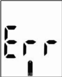
A square icon representing an error message. It features the letters 'Err' in a large, stylized, seven-segment font. Below the letters is a small, vertical bar with a notch at the top, resembling a test strip.        | <b>Humidified / Used strips</b><br>The meter has detected a problem with the test strip. | <b>Repeat the test with a new strip.</b><br>Refer to pages 27-28 for information on sample application. |
