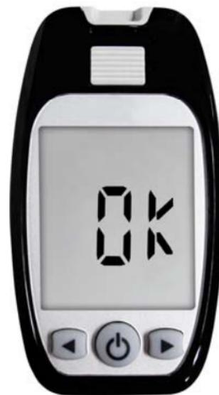
3. When all data are uploaded from the meter to the PC, the meter shows "OK" and beeps.
