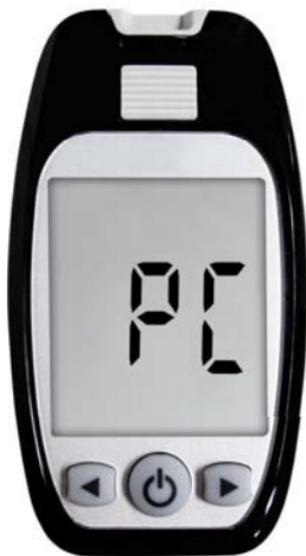
1. Use the USB cable to connect to the meter and your computer. The display shows "PC".
