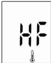
The “HF” and thermometer icon appears. Temperature is too high, outside the required range of 10°C - 40°C (50°F - 104°F). This alerts users that an incorrect result may occur if the test continues.
