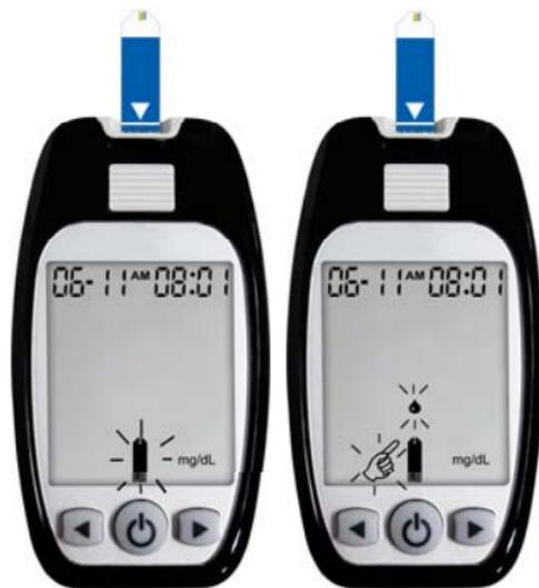
2. Put a test strip into the meter in the direction of the arrow. The meter turns on automatically. The icon shows itself.
