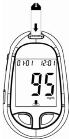
9. The meter starts to count down from 5 seconds and then shows the test result.
