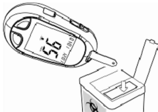
10. Push the Strip Ejector to remove the test strip.
