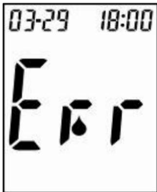
**Err message. Not enough sample was drawn into the test strip for measurement.**
