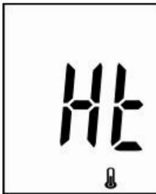
**The "Ht" and thermometer icon appears. Temperature is too high, outside the required range of 10°C - 40°C (50°F - 104°F). This alerts users that an incorrect result may occur if the test continues.**
