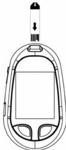
2. Put a test strip into the meter in the direction of the arrow. The meter turns on automatically.
