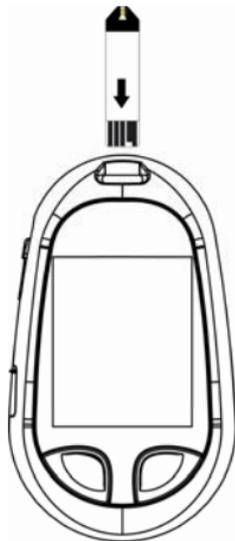
1. Put a test strip into the meter as the direction of the arrow on the test strip. The meter turns on automatically.
