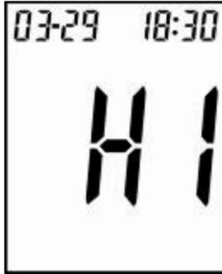
**Test result is higher than 630 mg/dL (35.0 mmol/L).**
