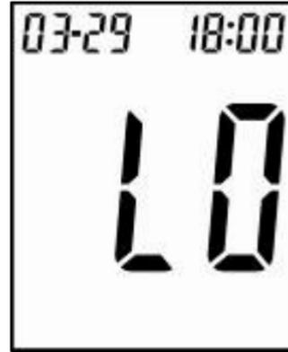
**The test result is lower than 20 mg/dL (1.1 mmol/L).**
