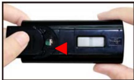
1. Open the battery door of the meter by slipping the tab in the direction of the arrow.
