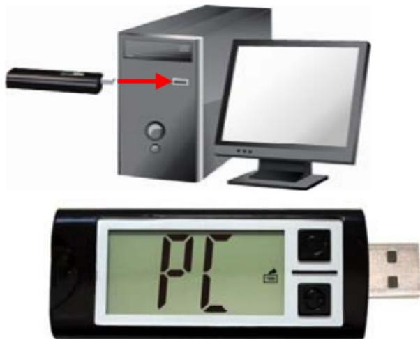
1. Plug the **EasyPlus mini MasterDriver™** meter into a USB port on your PC.
