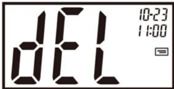
4. To delete a test result, press
