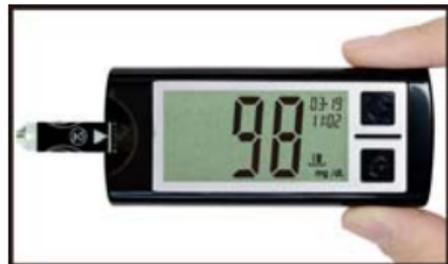
7. The meter starts to count down from 5 seconds, the display shows "Ok", and then shows the test result.
