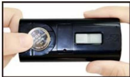
2. Insert a battery and the meter beeps.
