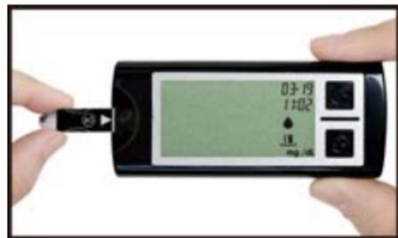
2. Put a test strip into the meter in the direction of the arrow.
