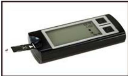
1. Put a test strip into the meter in the direction of the arrow.
